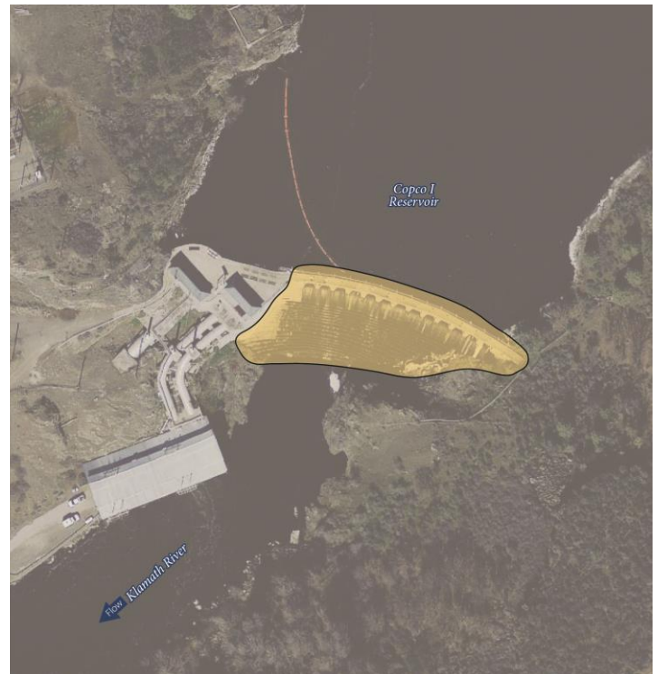
Figure ES-19: Partial removal of Copco 1 Dam would include removal of the concrete dam, providing a free flowing river and allowing full volitional fish passage. Certain structures, including the penstocks and powerhouse, would be retained.
