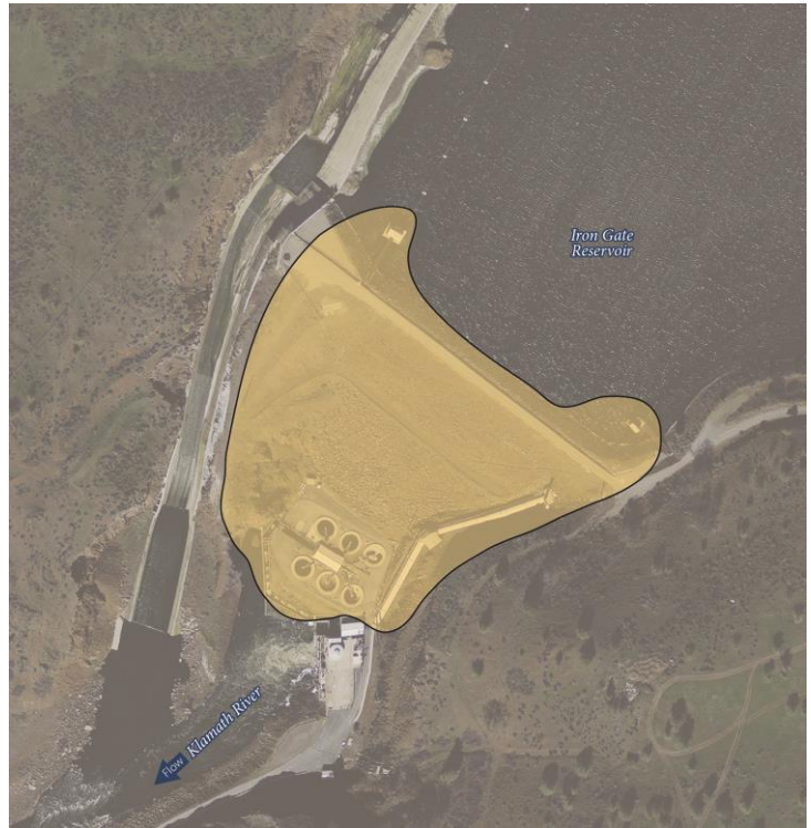
Figure ES-21: Partial removal of Iron Gate Dam would include removal of embankment dam, providing a free flowing river and allowing full volitional fish passage. Certain structures, including the spillway and powerhouse, would be retained.
