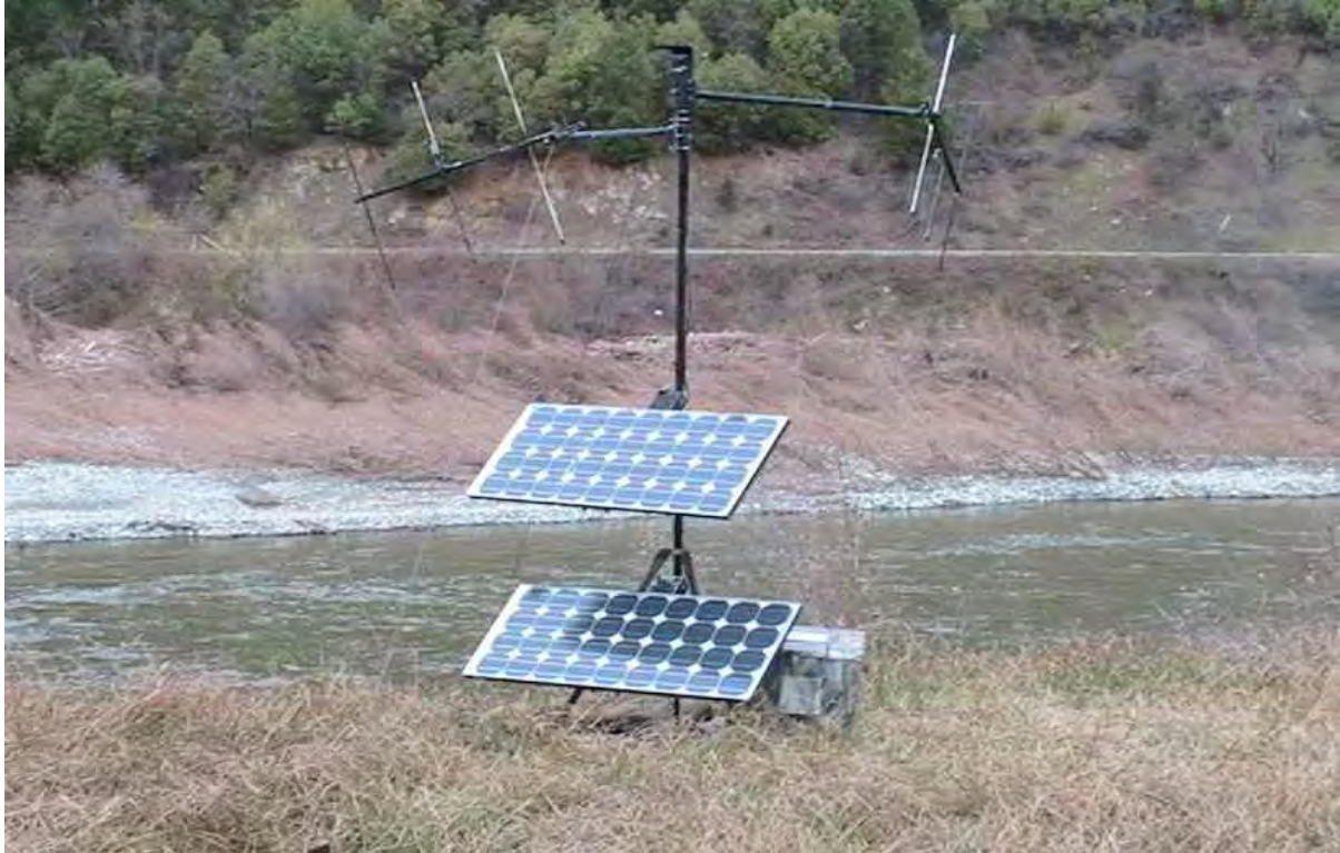
Figure 2. Photograph showing typical automated radio telemetry detection station. This site is located approximately 1.5 km upstream of the confluence between the Klamath River and Indian Creek, northern California.
