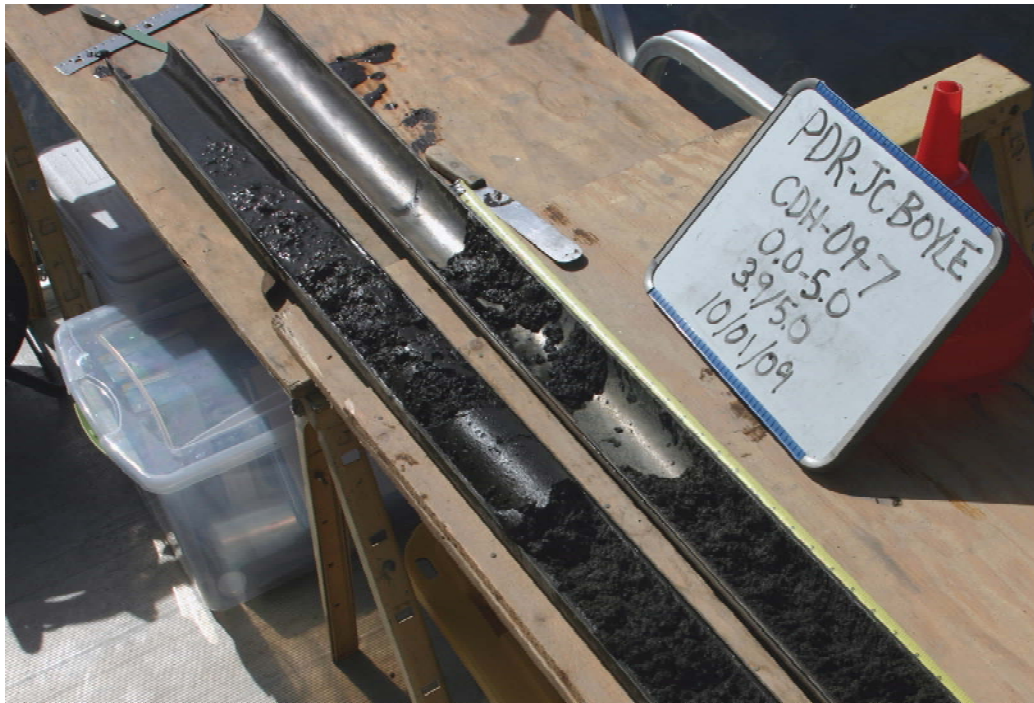
Figure 7 - Sediment sample within the FADC split tube.
