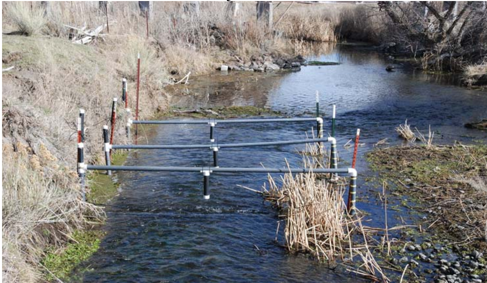
Photo 18. Directional Antenna System at HIG 1
