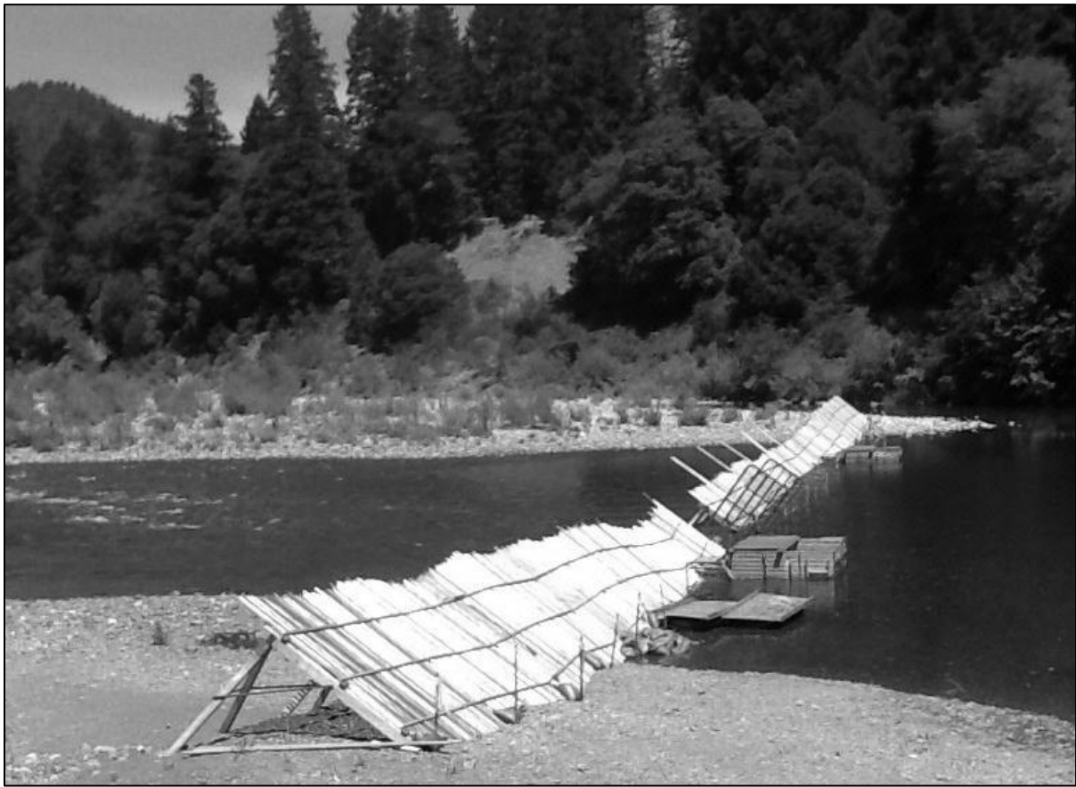
Figure 3. Set up of Willow Creek weir, 2013. Two trap boxes with a boat gate in between.
