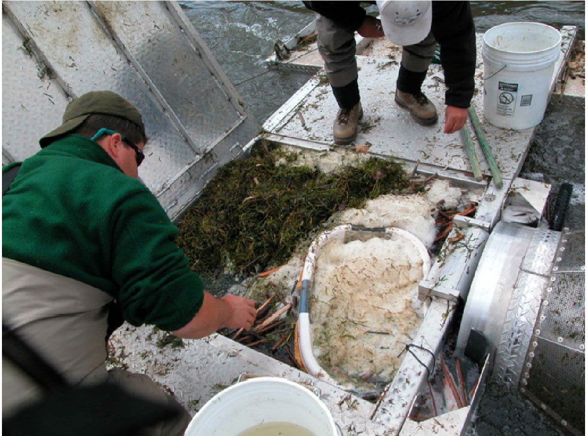
Figure III-8. Juvenile outmigration trap located below Iron Gate Dam, inundated with aquatic vegetation (2004 USFWS photo).
