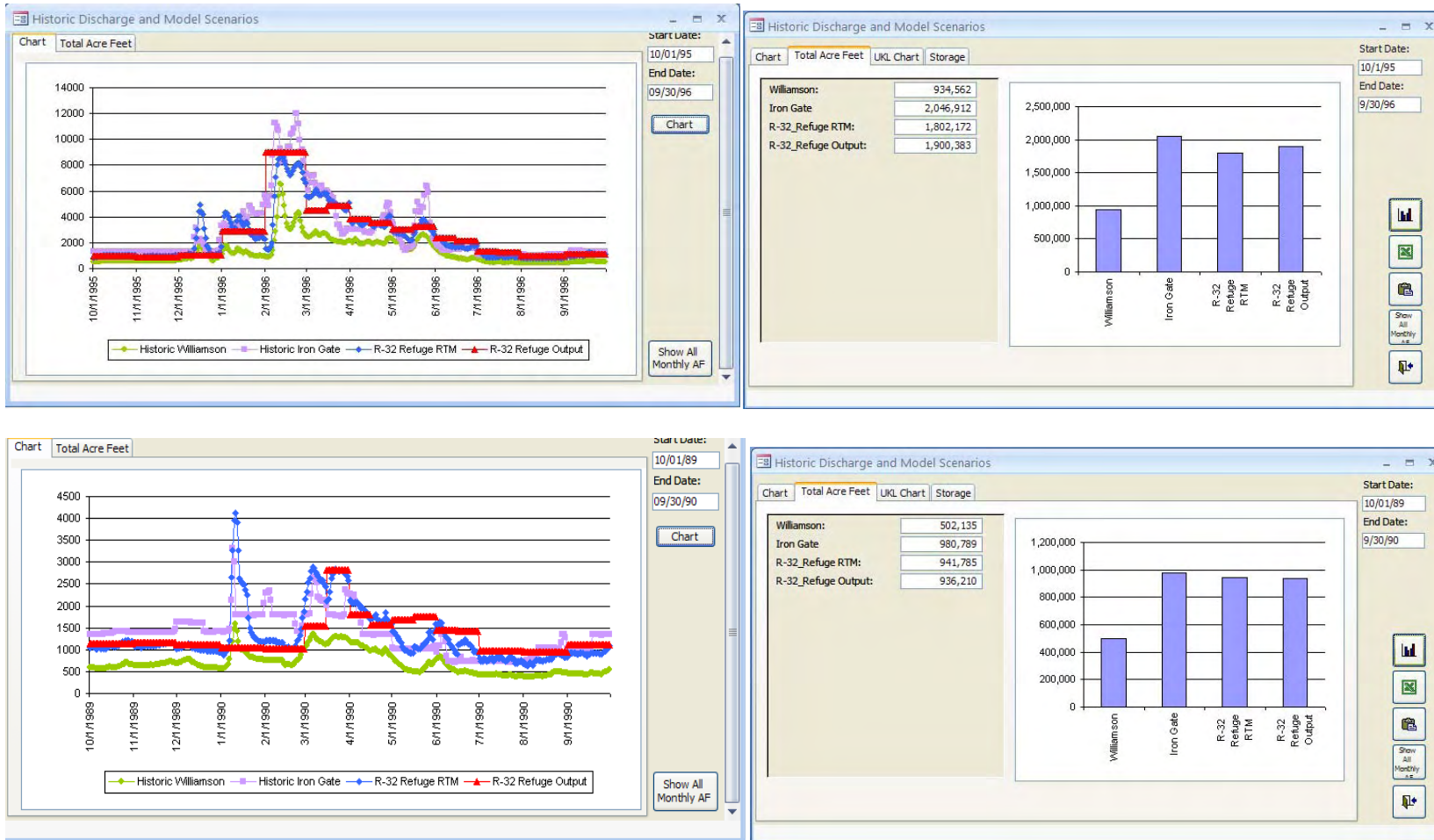
Figure VI-6. RTM database interface display comparing daily flows (left) and total annual discharge in acre feet (right) for the historical Williamson River, historical Iron Gate, Run-32 Refuge RTM, and Run-32 Refuge model outputs. The top charts represent an above average water year (1996), and the bottom charts represent a below average water year (1990).
