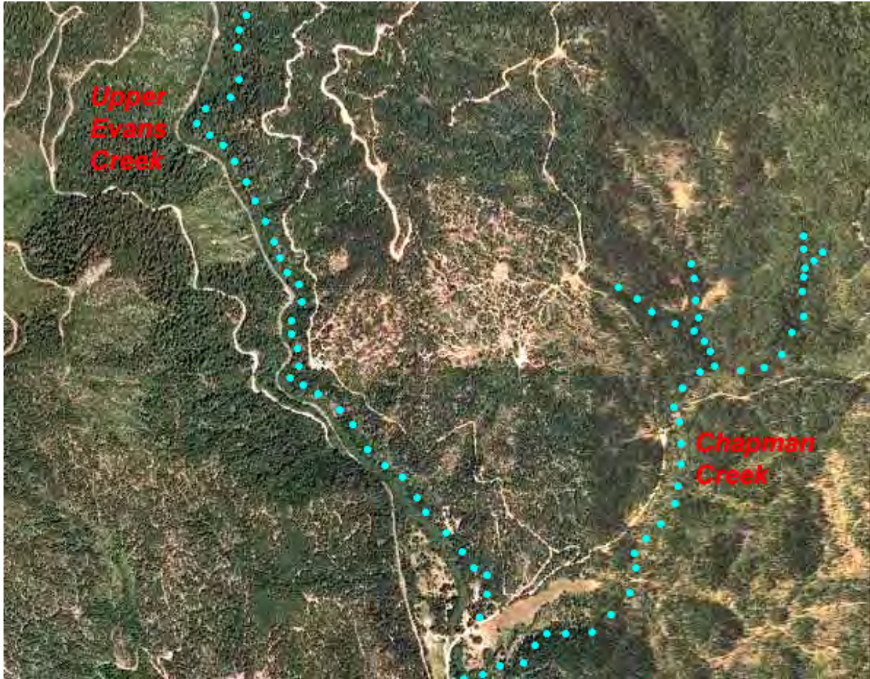
Figure 32-9. Upper Evans Creek and tributary Chapman Creek shown with dots. Timber management roads are immediately next to the channel and there is an extensive network of skid trails that can alter watershed hydrology and sediment yield. Stream courses are based on the USGS (1989) topographic map. June 2005.
