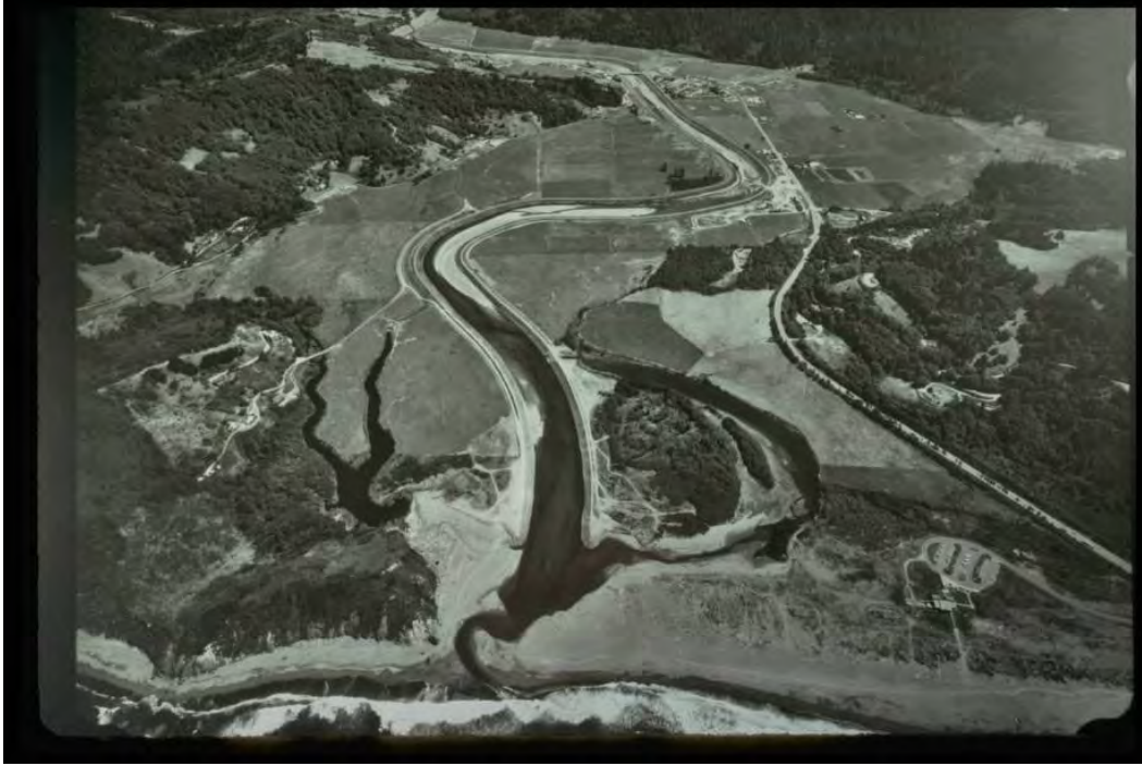
Figure 19-3. Aerial photograph of the Redwood Creek estuary, with levees. Photo shows the levees and continued gravel and vegetation removal for channel maintenance; note the much-reduced estuary size and reduction in habitat complexity. Redwood Creek estuary in 1988 from KRIS.
