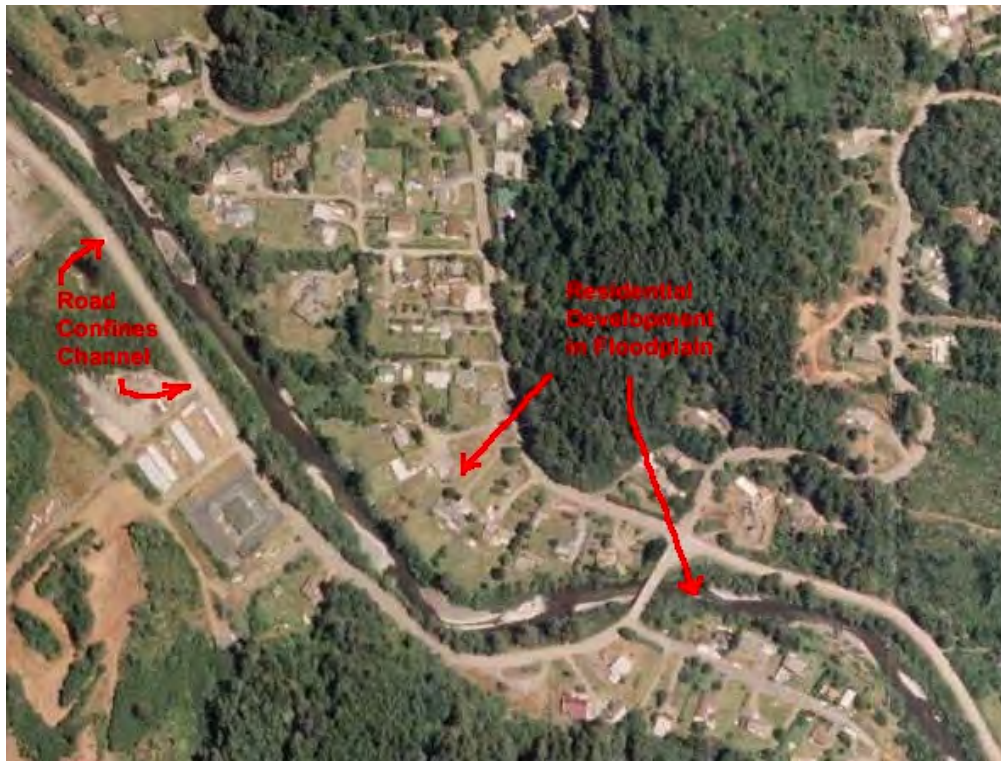
Figure 11-3. Lower Hunter Creek flows adjacent to residential development. Creek is closely confined by a berm for Hunter Creek Road. Some houses encroach closely upon the creek and fully occupy the riparian floodplain.
