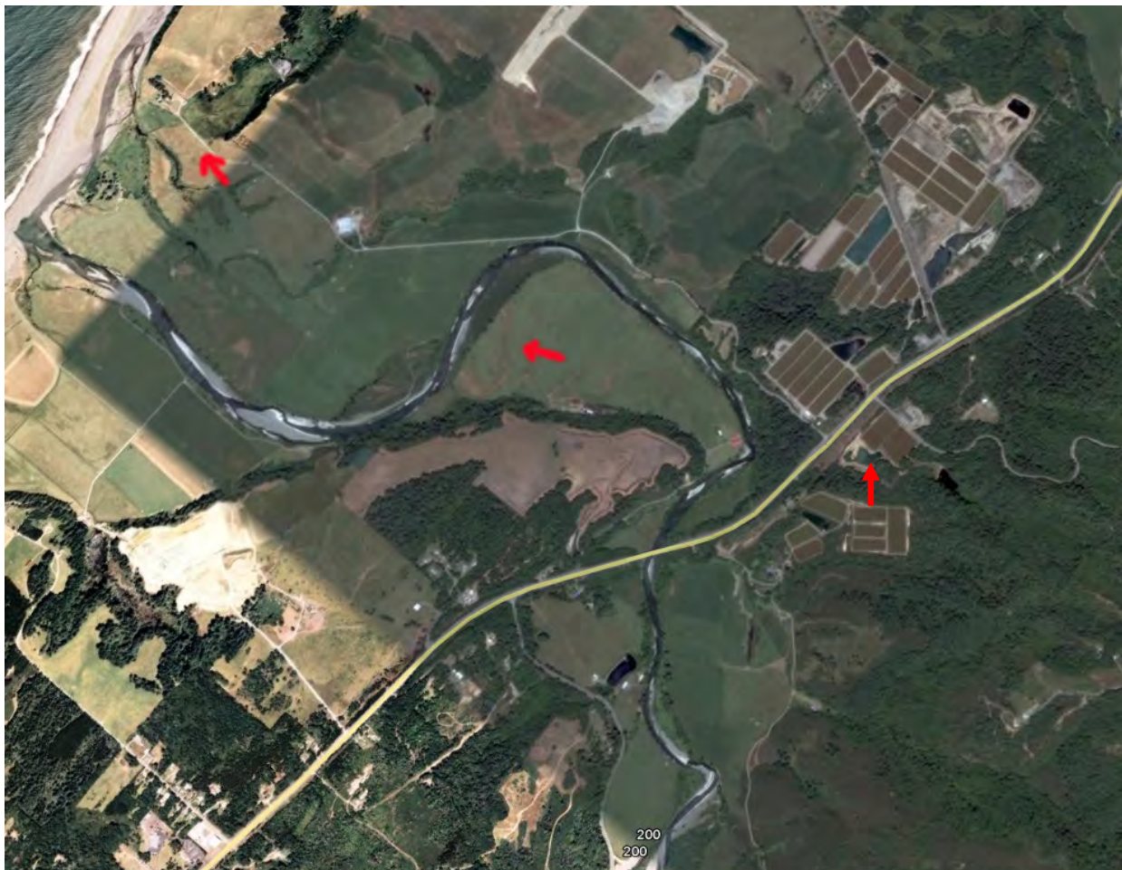
Figure 7-2. Aerial image from Google Earth of the Lower Elk River above and below Highway 101 (yellow line is highway). Rectangular beige shapes are cranberry bogs. Filled river meanders, cutoff wetlands and streams, and an irrigation pond on a tributary (right) are highlighted with red arrows.
