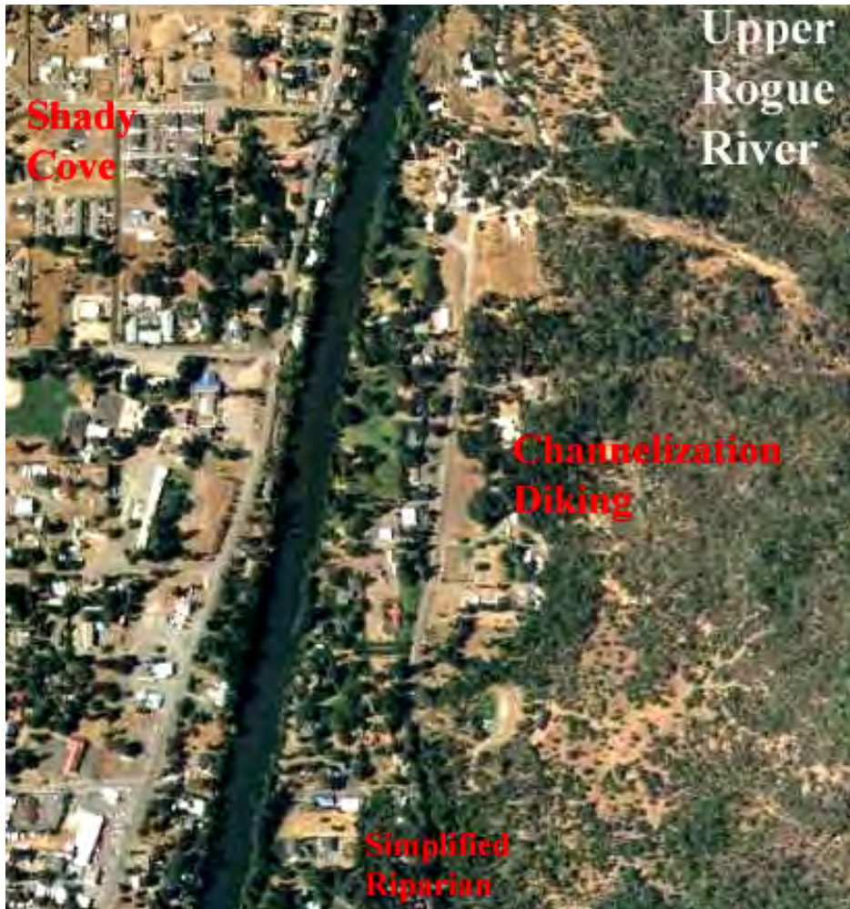
Figure 32-7. The Upper Rogue River running through Shady Cove. This 2005 aerial photo shows channelization, lack of a functional riparian vegetation, and potential risk of non-point source pollution.
