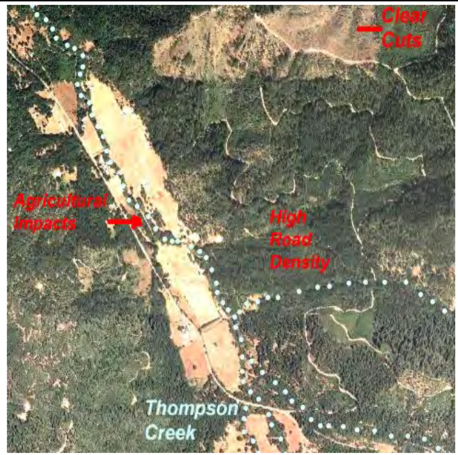
Figure 30-9. Aerial photo showing very high road densities in upper Thompson Creek. All of upper Deer Creek, which includes Thompson Creek, has a road density of 4 mi./sq. mi. Photo from 2005.
