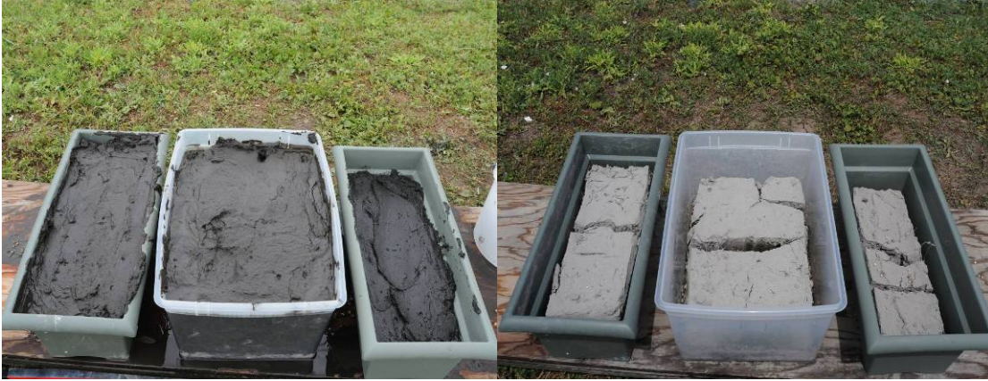
Figure 5.8. Picture of sediment from JC Boyle immediately after placement (left) and 15 days after placement (right).
