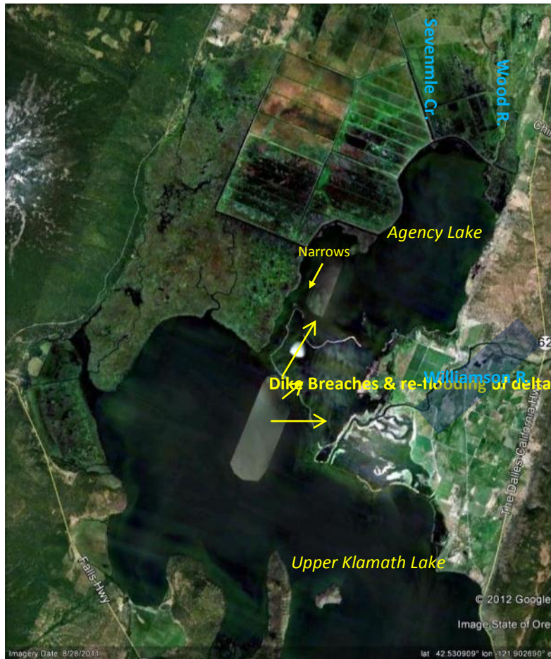
Figure 11. Wetland restoration activities on the Williamson River Delta allowing for greater connectivity between Agency Lake and Upper Klamath Lake.
