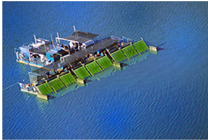
Figure 26. In situ algae harvesting barge. Note nine screen panels which rotate through water column to capture algae. Mechanical rakes then remove algal biomass and shunt algae to holding tanks within the barge. Source: Simplexity Health Inc.
