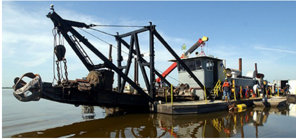
Fig. 2.22 A typical hydraulic dredging operation. Photo: www.naplesnews.com.
