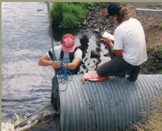
Fig. 1.19 Klamath Tribe water quality technicians measuring pumped discharge from the Wood River Ranch into Sevenmile Creek; circa 1992. Photo: Jacob Kann.
