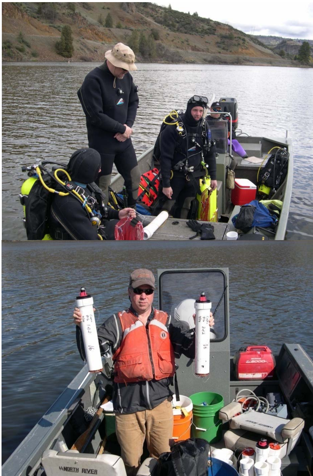
Figure 4. Sediments collected by SCUBA using 3-in by 8-in push tubes, with samples capped at depth to prevent oxidation, and stored upright on ice for transportation to laboratory, April 2010.
