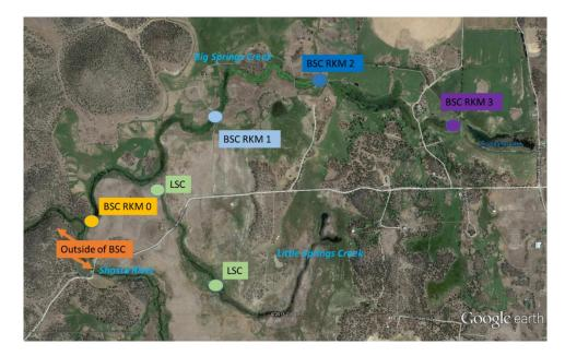
Figure 18.PIT tag antenna stations in Big Springs and Little Springs Creeks.
