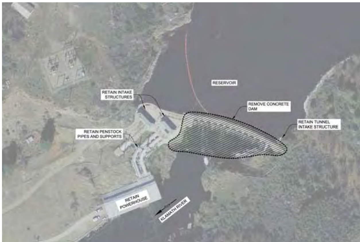
Figure 2-17. Copco 1 showing portion of dam to be removed for the Partial Facilities Removal Alternative.
