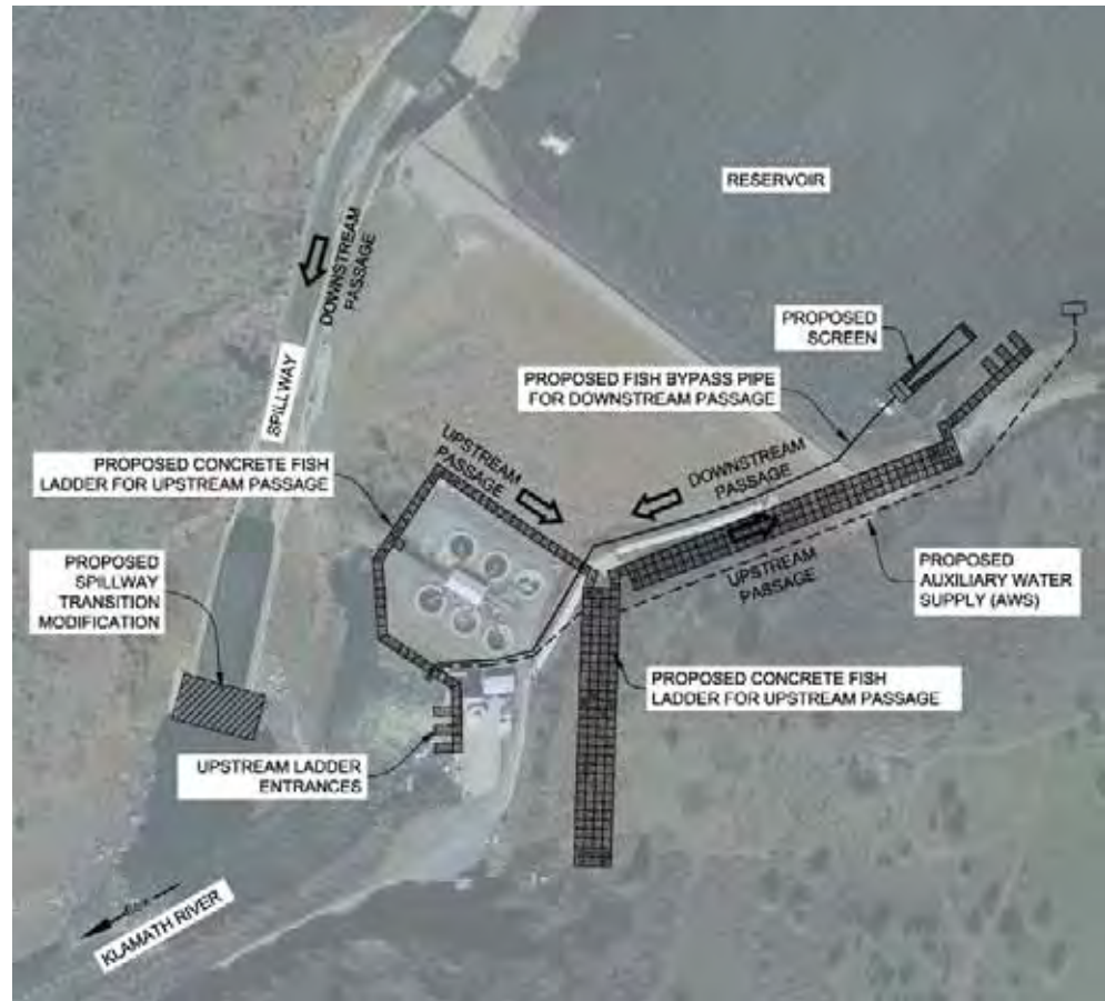
Figure 2-27. Conceptual fish passage facilities layout for Iron Gate Dam showing fish ladder, water intake screen, and spillway transition modifications.
