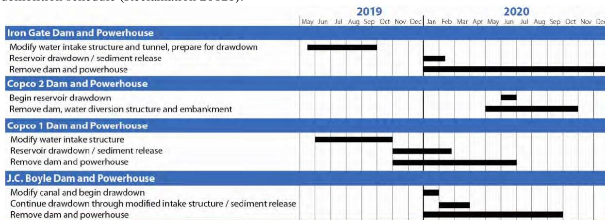
Figure 2-2. Anticipated Schedule for Full Removal of the Four PacifiCorp Dams and Facilities
