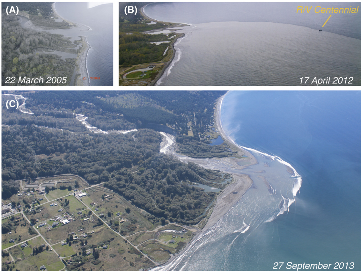
Fig. 7. Oblique aerial photos of the Elwha River mouth before and during dam removal. Photos show (A) the river mouth wetlands before dam removal, (B) the turbid buoyant coastal plume that occurred during much of the dam removal project, and (C) the expansion of the river mouth delta by \sim 2.4 million \text{m}^3 of sediment deposition. The R/V Centennial shown in (B) is 18 m in length. Photos provided by Ian Miller of Washington Sea Grant, Jonathan Felis of USGS, and Neal and Linda Chism of LightHawk.
