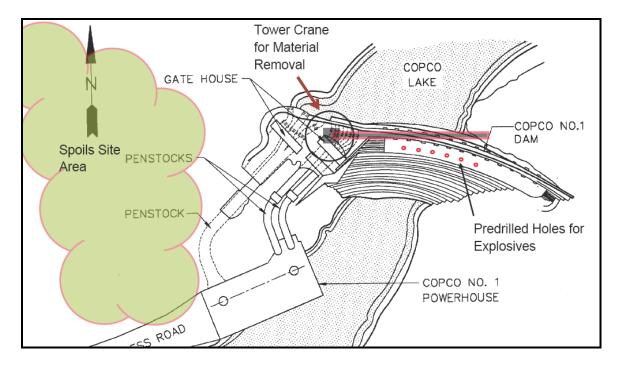
Figure 34 Copco 1 Dam Demolition Approach
