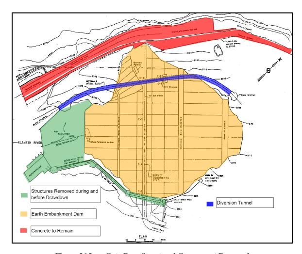
Figure 26 Iron Gate Dam Structural Component Removed
