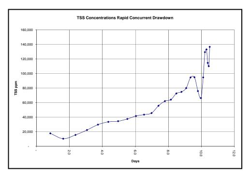
Figure 17 TSS Downstream of Iron Gate for Concurrent Rapid Drawdown
