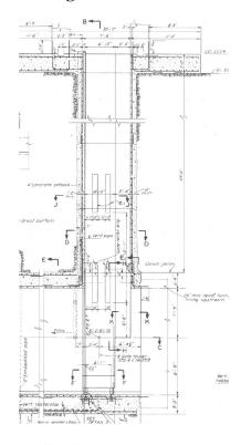
**Figure 24 Section through Upstream Gate**
