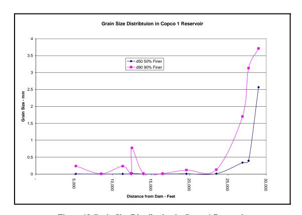
Figure 12 Grain Size Distribution in Copco 1 Reservoir
