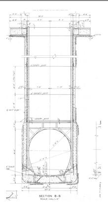
Figure 23 Section through Diversion Tunnel at Upstream Gate
