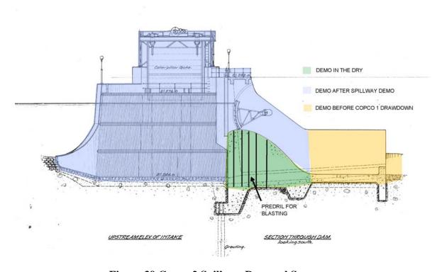
Figure 39 Copco 2 Spillway Removal Sequence
