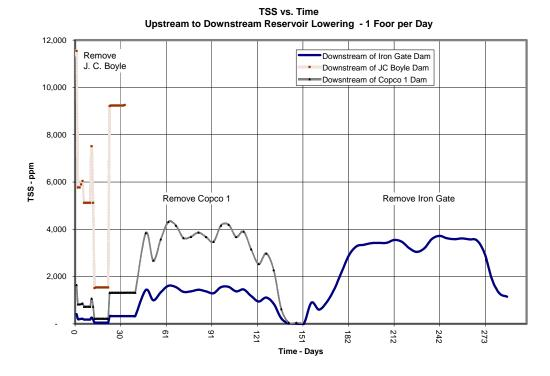
Figure 15 TSS Resulting from Upstream to Downstream Removal
