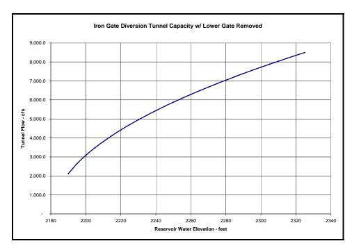
Figure 21 Iron Gate Tunnel Capacity Fully Open
