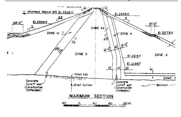
**Figure 27 Section through Iron Gate Dam**
