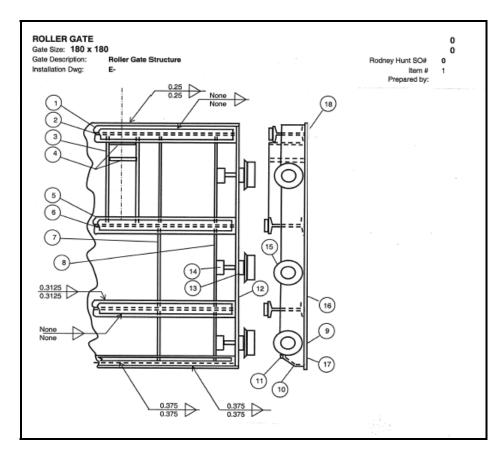
Figure 22 Partial Elevation and Section of Downstream Control Gate
