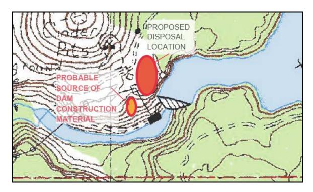
Figure 33 Plan View of Copco 1 Dam and Proposed Spoils Site
