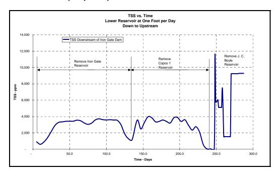
Figure 16 Downstream to Upstream Removal
