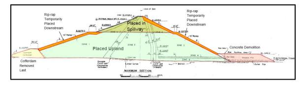
Figure 25 Section Through Iron Gate Dam Showing Excavated Material Site Placement
