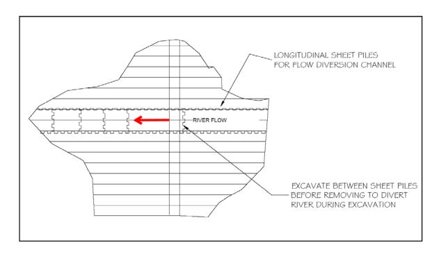
Figure 28 Iron Gate Cofferdam Removal
