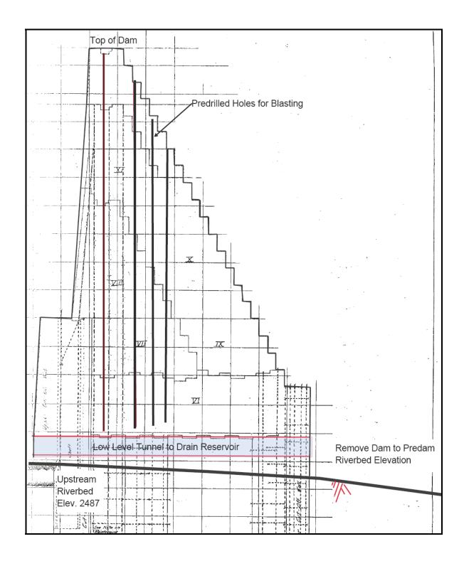
Figure 36 Section Through Dam Showing Removal Approach
