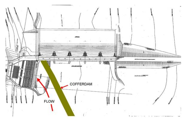
Figure 41 Cofferdam Diversion at Copco 2
