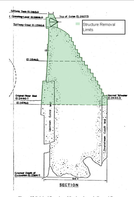
Figure 35 Original Drawing of Section through Copco 1 Dam
