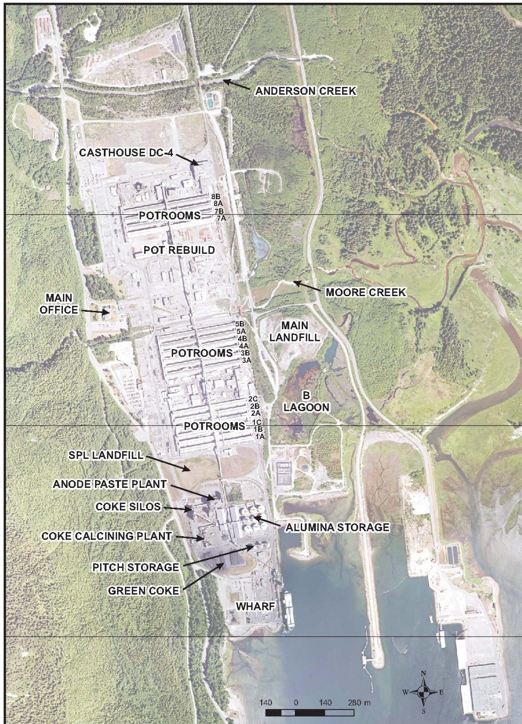
Figure 2.2-1: Site plan: existing smelter components.
