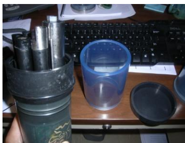
Figure 22. Calibration cup with black covering used for calibration procedure.
