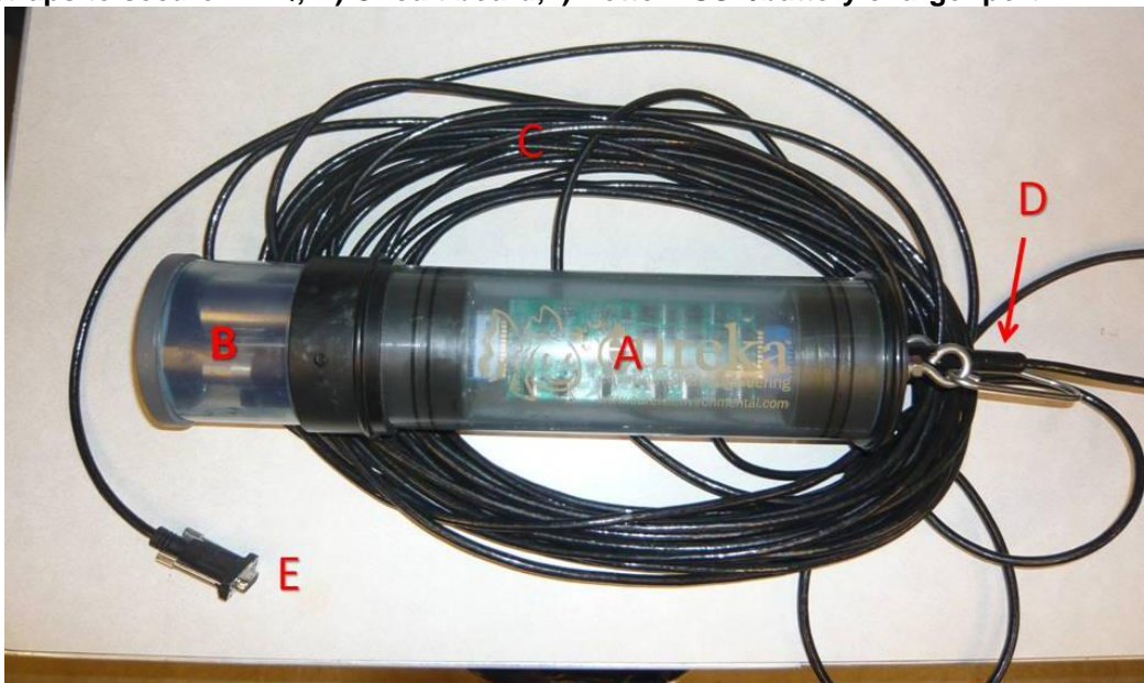
Figure 16. Manta overview. Manta parts: A) Manta body; B) Storage cup; C) 25 m cable; D) Waterproof, integral cable connection; E) Marine-grade serial port.
