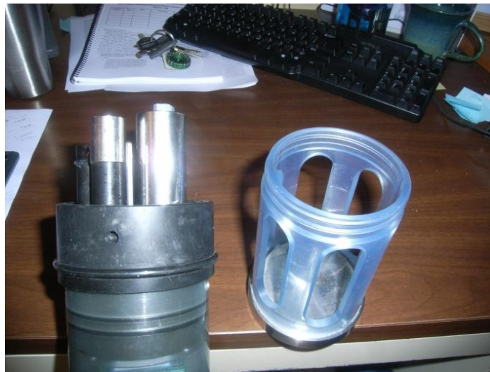
Figure 21. After removal of storage cup, weighted cup on left is attached by screwing into the Manta body. Note that the weight is heavy and exerts leverage. Use a firm grasp so that the weighted cup does not interfere or break any of the probes.
