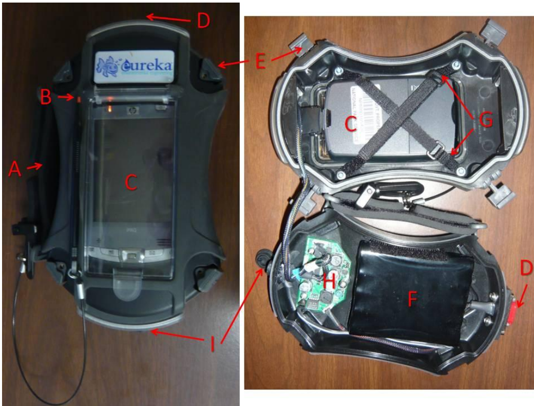
Figure 15. Amphibian overview – top down (Left); open (Right). Amphibian parts: A) Neoprene handle; B) Stylus; C) iPAQ pocket PC; D) Top serial port; E) Case clasps; F) External battery; G) Velcro straps to secure iPAQ; H) Circuit board; I) Bottom USB/battery charger port.
