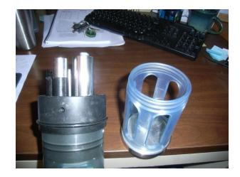
Figure 2. After removal of storage cup, weighted cup on left is attached by screwing into the *Manta* body. Note that the weight is heavy and exerts leverage. Use a firm grasp so that the weighted cup does not interfere or break any of the probes.
