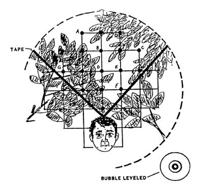
**Figure 5.** Schematic of modified convex spherical canopy densiometer (from Mulvey et al.1992). In this example, 10 of the 17 intersections show canopy cover, giving a densiometer reading of 10. Intersections not showing canopy cover are indicated with letters A-G. Note proper positioning with the bubble leveled and face reflected at the apex of the "V."
