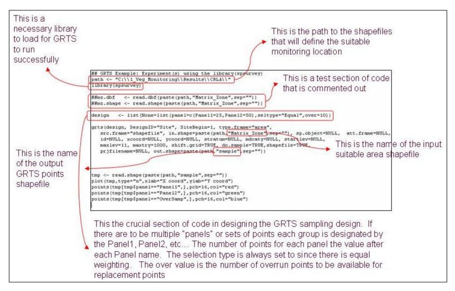
Figure 8. Layout of GRTS code to be run in the Software "R."
