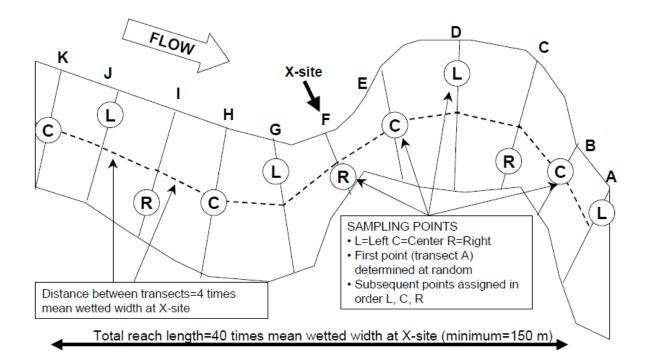
Figure 31. Schematic overview of the reach layout, showing the "X" point at the F transect and the center of stream line used to measure the distance between transects. From EMAP Western Pilot Study Field Operations Manual.
