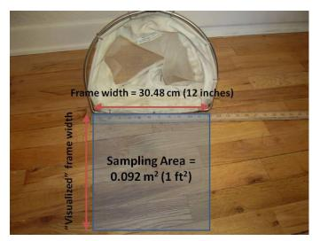
Figure 39. Example D-frame kicknet used for macroinvertebrate collection.
