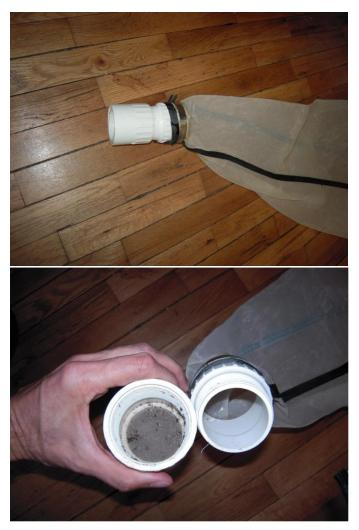
Figure 40. Dolphin bucket (top – attached; bottom – unscrewed for dumping) at end of invertebrate sampling net (if so equipped).
