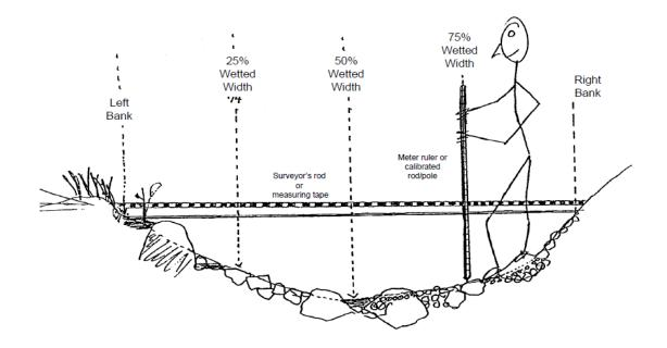
Figure 47. Cross-section schematic showing substrate measurement details.
