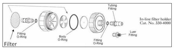
Figure 38. Diagram of inline filter holder (NALGENE<sup>®</sup>) showing assembly. In this configuration, the input is on the right (use the Luer fitting) and the outflow is on the left.
