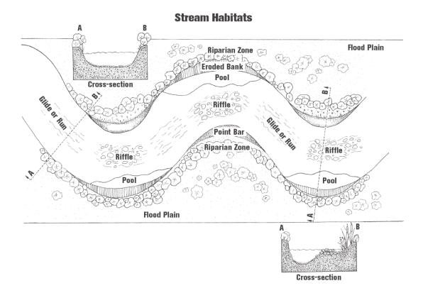
Figure 41. Potential discharge measurement channel cross section placements within a stream. The cross-section on the left has the ideal qualities for the measurement of discharge. The cross-section on the right has an irregular depth profile, substrates that cause turbulent flow, and aquatic vegetation near the bank, therefore making it an unacceptable channel cross-section for the measurement of discharge (from TCEQ 2008).
