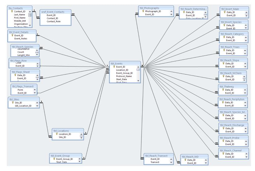
Figure 63. Relational diagram of the tables contained in the KLMN stream monitoring database.
