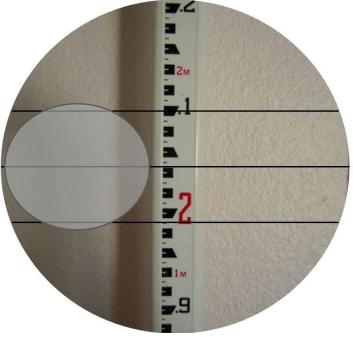
Figure 49. An approximate view through the Abney Level. The bubble on the left indicate levelness using the upper and lower lines. The reading is taken using the middle line as accurate as possible.
