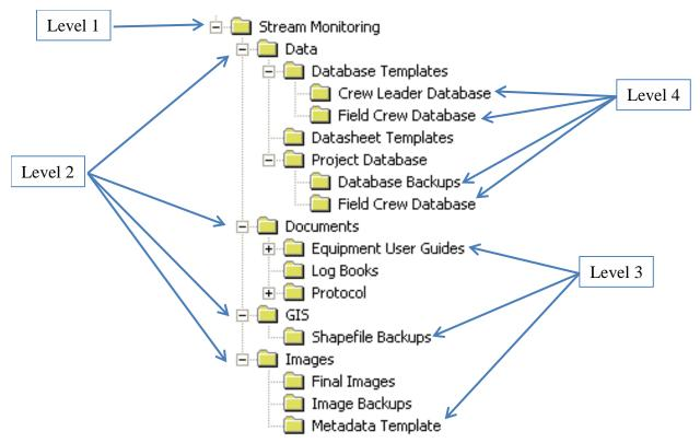
Figure 10. File structure used on tablet computers to support the stream monitoring protocol.
