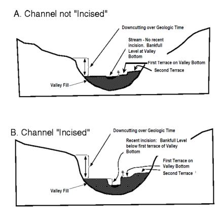
Figure 48. Schematic showing bankfull channel and incision for channels. (A) not recently incised, and (B) recently incised into valley bottom. "Recent incision" indicated on (B) is the distance to be measured and recorded as "incised height" on the field data form. Note level of bankfull stage relative to elevation of first terrace on valley bottom (stick figure included for scale).
