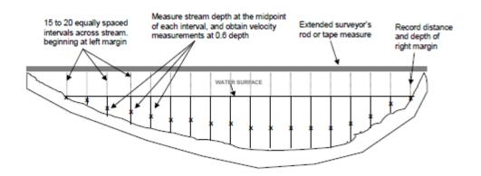
Figure 42. Diagram of placement of cross-sectional measurement for velocity.
