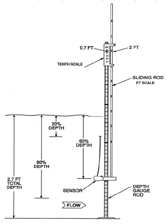
Figure 43. Diagram of the wading rod. In this example, the depth is 2.7 ft, and when the sliding rod is set at 2.7; the sensor is automatically at 60% of the water depth.
