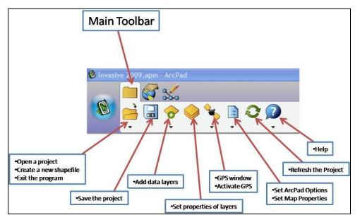
Figure 32. Description of functions available in ArcPad using the main toolbar.
