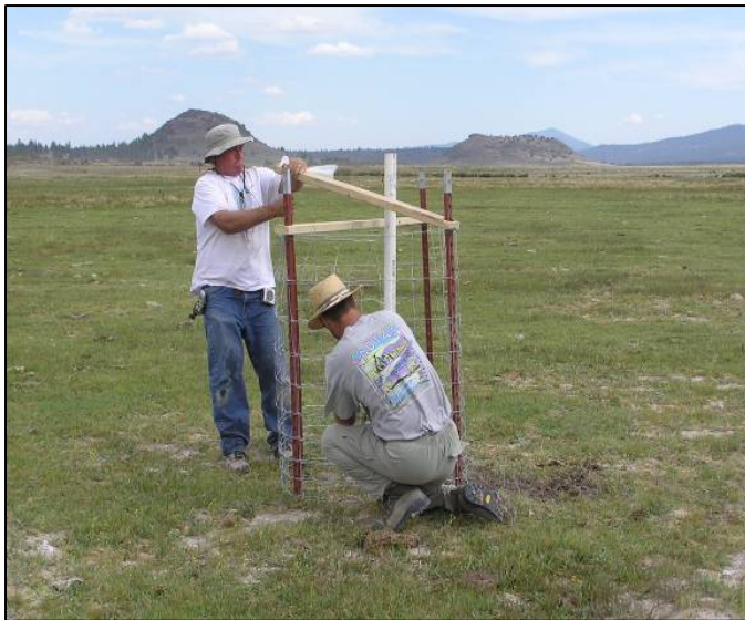
Figure 10. Photo of the Installation of a Piezometer to Measure Water Table Levels.
