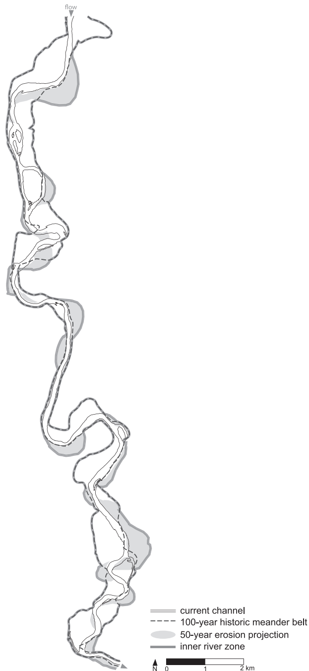
Figure 6. The “inner river zone” of the Sacramento River Conservation Area from approximately km 215 to km 255. This zone (in which the river is proposed to be allowed to migrate freely except at infrastructure) was determined from channel migrations over the preceding century (based on analysis of historical maps back to the 1890s and aerial photographs) and projected channel migration for the coming 50 years (based on modeling). Unpublished GIS data layers courtesy of the California Department of Water Resources, Red Bluff.
