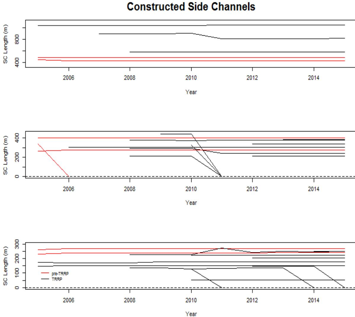
Figure B-2. Length of constructed side channels over the study period, 2005-2015. Side channel length is depicted by a line for the years the side channel is either visibly connected (>0) to or temporarily disconnected (= 0) from the mainstem Trinity River over the study period as determined by visual inspection of aerial photographs. Note, to aid visualization, constructed side channels are displayed in three panels and the y-axes are not scaled the same.
