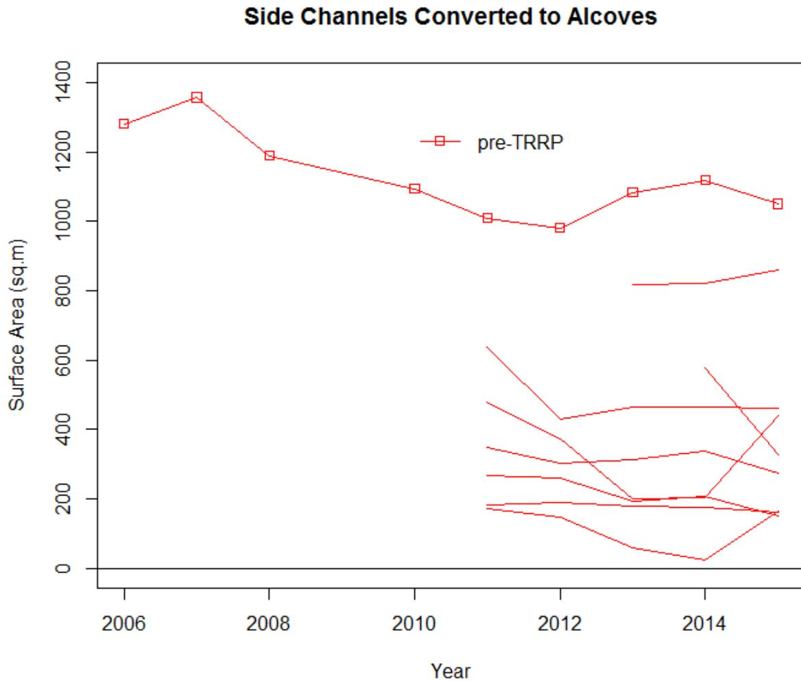
Figure B-4. Surface area of side channels that converted to alcoves over the study period, 2005-2015. Alcove surface area is depicted by a line for the years the alcove is visibly connected to the mainstem Trinity River over the study period as determined from visual inspection of aerial photographs. One converted side channel constructed prior to the TRRP (pre-TRRP) is at the top of the figure.
