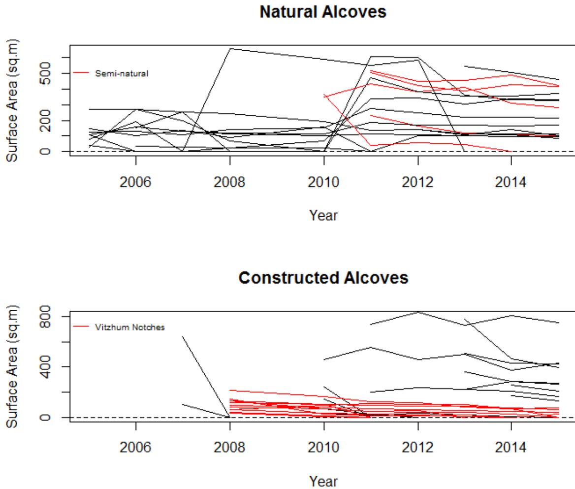
Figure B-3. Surface area of constructed and natural alcoves over the study period, 2005-2015. Alcove surface area is depicted by a line for the years the alcove is visibly connected to the mainstem Trinity River over the study period as determined from visual inspection of aerial photographs. Semi-natural alcoves that formed as a result of gravel augmentation activities (upper panel) and Vitzhum notches (lower panel) are in red. Note the y-axes are not scaled the same to aid visualization.
