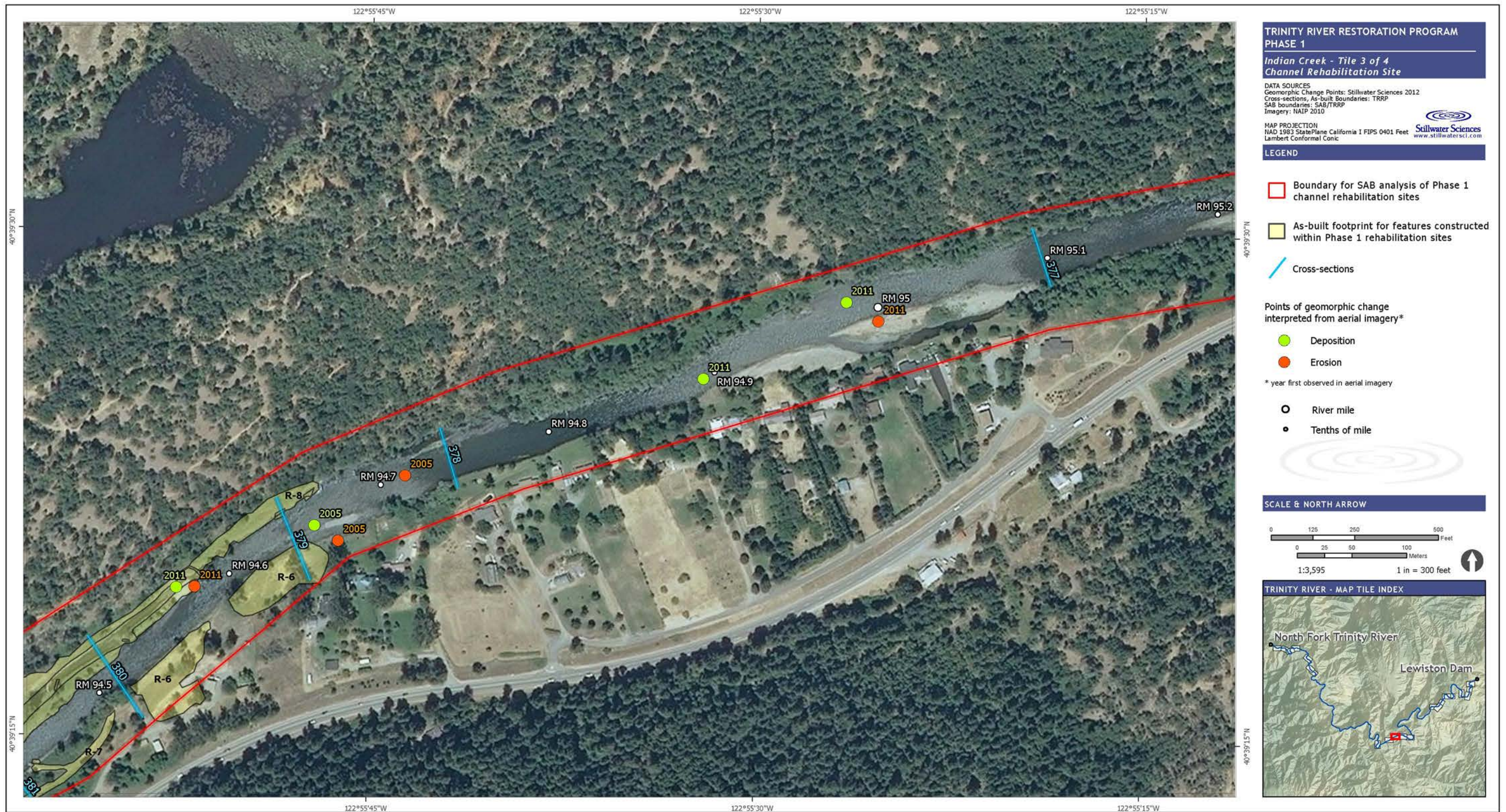
Figure 6-13c Design Features at the Indian Creek Rehabilitation Site, including Cross Sections Analyzed for Active Bed Width, Erosion, and Deposition Observed in Aerial Photography
