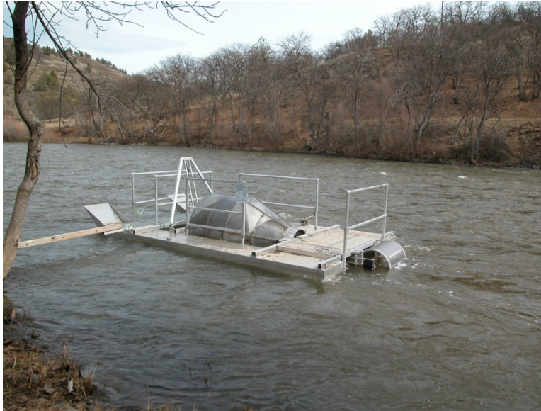
Rotary screw trap used to monitor the abundance of outmigrant juvenile salmonids on the Klamath River near Bogus Creek.
