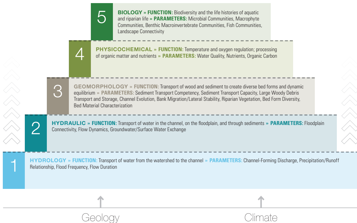
FIGURE 4.2 STREAM FUNCTIONS PYRAMID — FUNCTIONS & PARAMETERS (See Appendix A for full-size version.)
