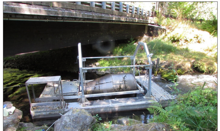
Figure 5. Screw trap used to monitor salmonid smolt outmigration in Indian Creek. (Photo by Mary Moser)
