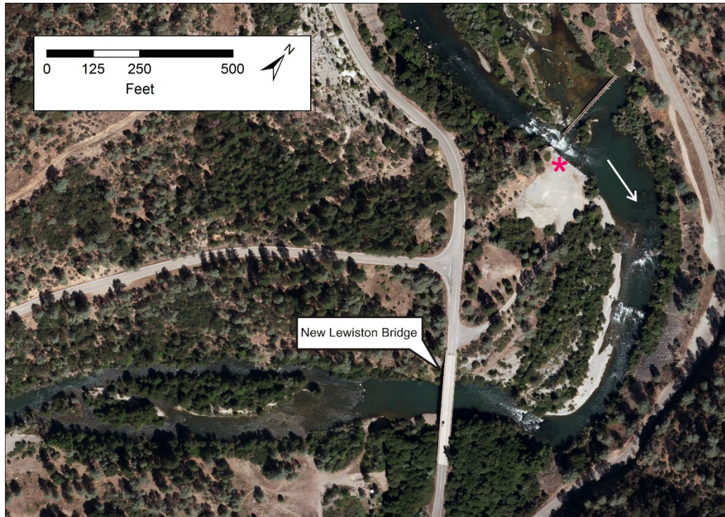
Figure 4: 2015 aerial photograph of the Diversion Pool reach of the Trinity River. The red asterisk indicates the gravel injection point and the white arrow indicates flow direction.
