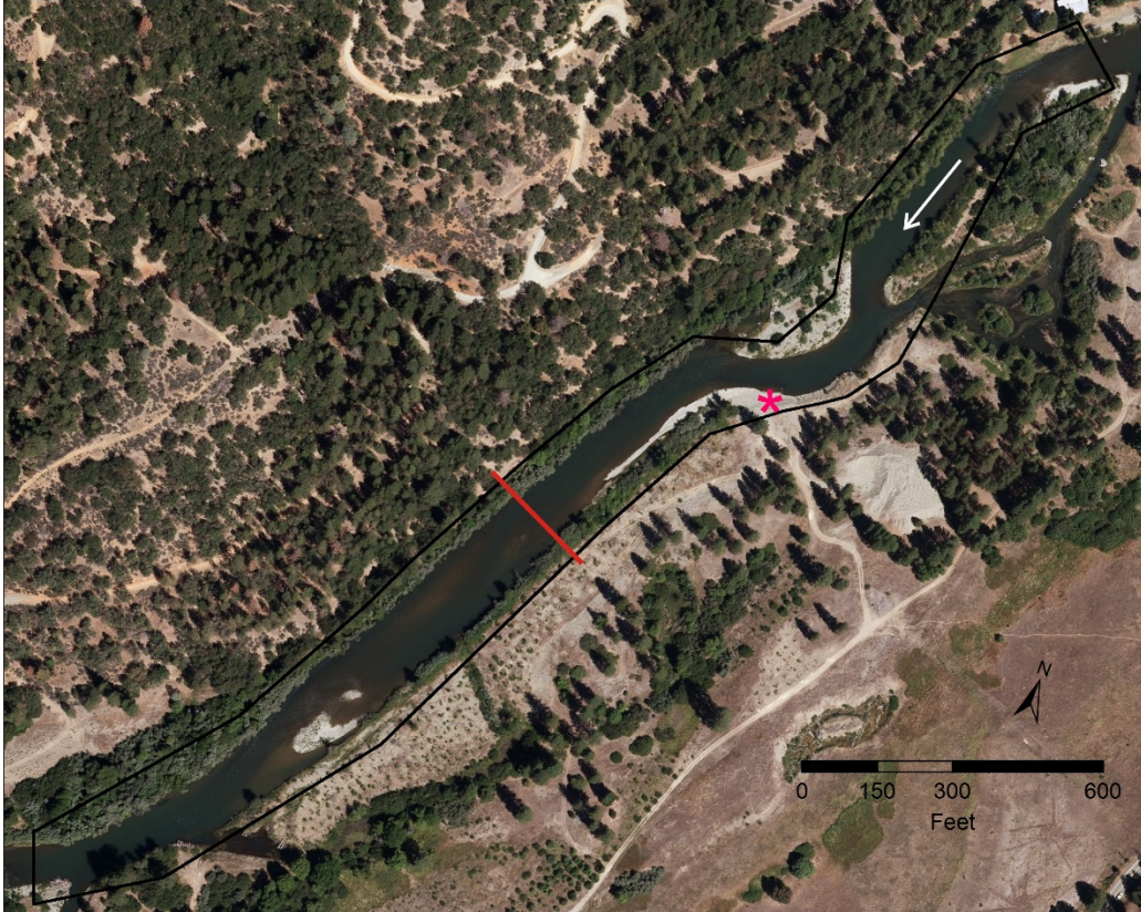
Figure 5: 2015 aerial photograph of the Lowden Ranch reach of the Trinity River. The section of channel surveyed with multibeam sonar in 2015 is outlined in black. The red asterisk indicates the gravel injection point, the red line indicates the sediment transport sampling transect, and the white arrow indicates flow direction.
