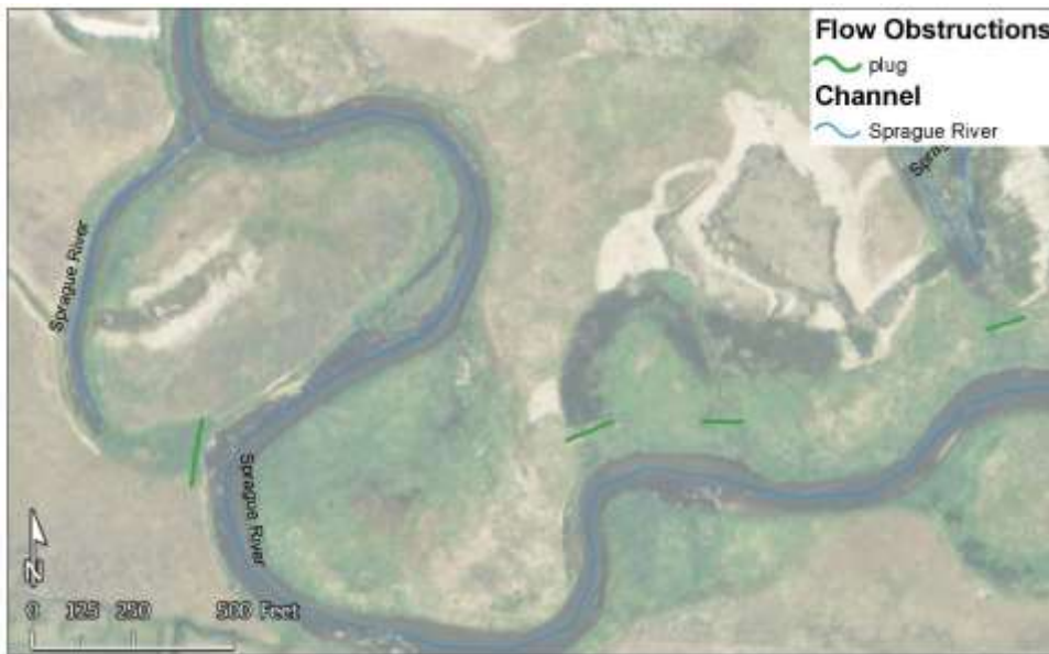
FIGURE 10: EXAMPLE OF PLUG FEATURES DELINEATED AT A RESTORATION SITE ALONG THE SPRAGUE RIVER.
