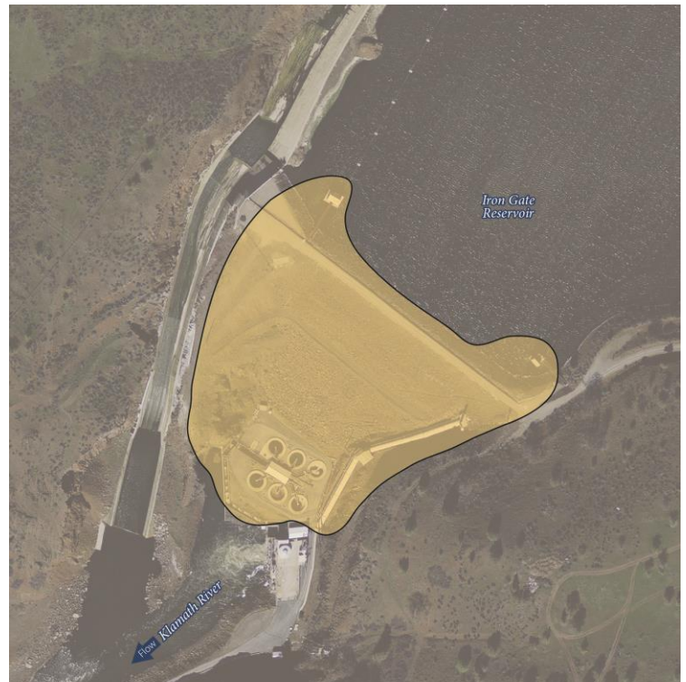
Figure 4.2-19: Partial removal of Iron Gate facility would provide a free flowing river and allow full volitional fish passage. However, certain structures would be retained or retained and buried.
