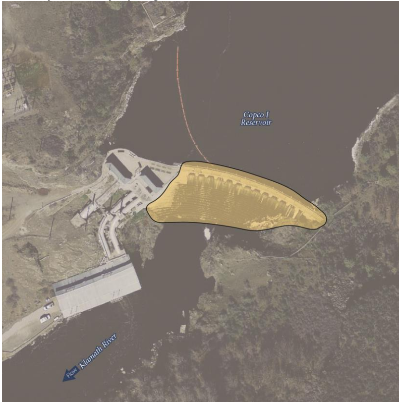
Figure 4.2-10: Partial removal of Copco 1 facilities would provide a free flowing river and allow full volitional fish passage. However, certain structures would be retained.
