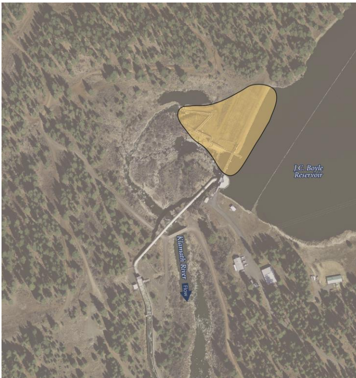
Figure ES-18: Partial removal of J.C. Boyle Dam would include removal of embankment dam and fish ladder, providing a free flowing river and allowing full volitional fish passage. However, certain structures, including the steel pipeline and supports, would be retained.
