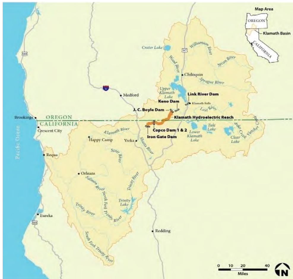
Figure 1-2: Klamath River Basin and PacifiCorp’s Four Facilities. The Klamath Basin covers over 12,000 square miles and includes PacifiCorp’s J.C. Boyle, Copco 1, Copco 2, and Iron Gate dams on the main stem of the Klamath River. These Four Facilities would be removed under the KHSA.
