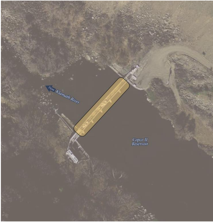
Figure ES-20: Partial removal of Copco 2 Dam would include removal of spillway gates, providing a free flowing river and allowing full volitional fish passage. Certain structures, including the water intake and embankments, would be retained.
