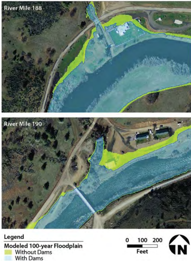
Figure 4.2-23: Close up of one or two structures potentially affected by the change in the 100-year floodplain – comparison of dams in and dams out floodplain. (NOT A REGULATORY FLOOD PLAIN, this is just a comparison)
