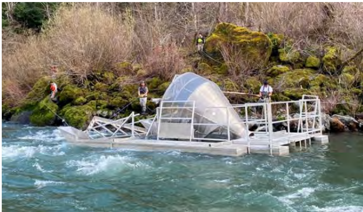
Figure 12. Juvenile outmigrant rotary screw trap (photo provided by Mike Belchik).
