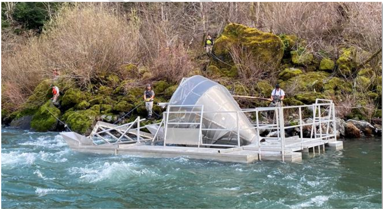
Figure 11. Juvenile outmigrant rotary screw trap (photo provided by Mike Belchik).
